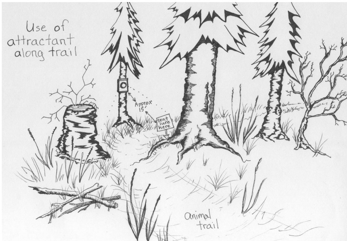
Figure 8. Remote camera trap set along a game trail incorporating a scent lure. Note the camera is looking down the trail rather than just across it. This should increase the amount of time an animal ends up in the view of the camera. Illustration by Jenn Wolfe.
