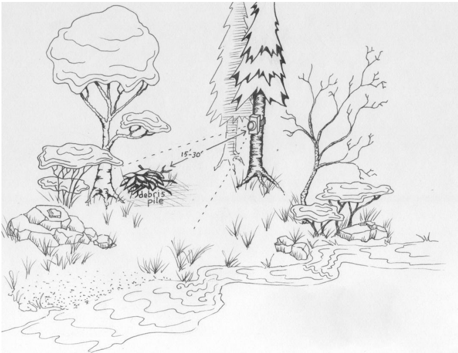
Figure 1. Layout of camera trap set. Illustration by Jenn Wolfe.
