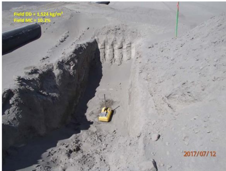
Photo II-5 Field Density Test Using Nuclear Densometer on the East Dam crest, inside excavated test pit, 1.2 m below the ground surface (ND17-ED-20)
