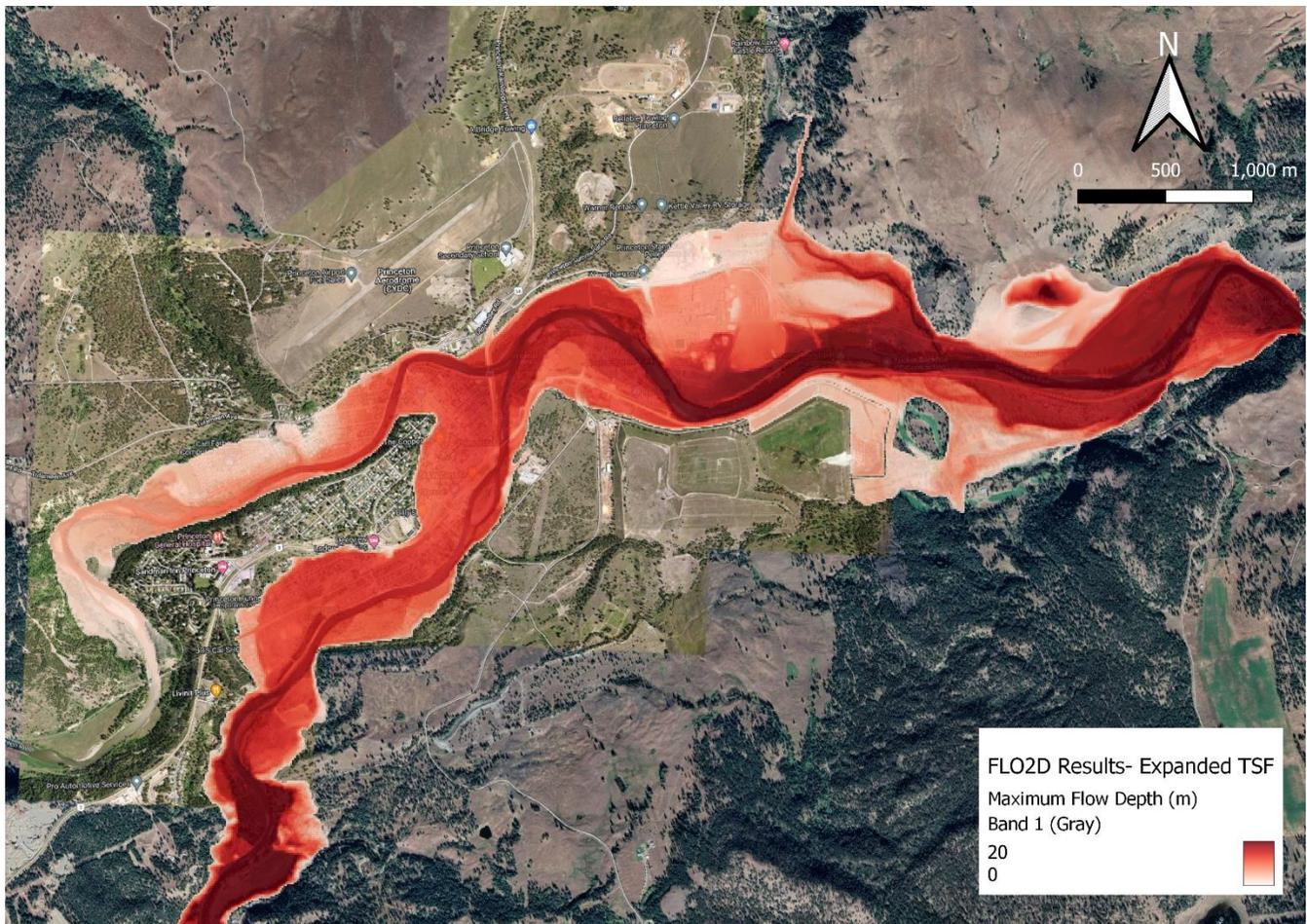
Figure 4-5: Maximum flow depths (m) in Princeton, BC from a 40% breach, 12 hour duration scenario for the expanded TSF at CMM (450 Mm<sup>3</sup>).
