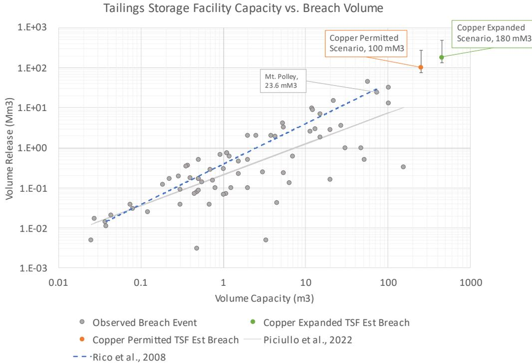
**Figure 2-2. Comparison of tailings storage facility capacity and observed release volumes for historical breach events. Calculated release volume scenarios used in this study (orange and green points) are derived from the Rico et al., (2008) regression line, since Piciullo et al. (2022) was published concurrent with our modeling efforts.**
