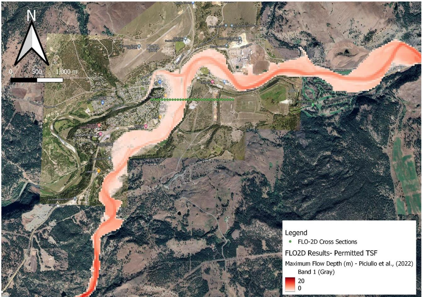
**A 24: Maximum flow depths (m) in Princeton, BC from a 15.0 Mm<sup>3</sup> breach, 12 hour duration scenario for the permitted TSF at CMM (250 Mm<sup>3</sup>), as predicted by Equation 1 in Piciullo et al., (2022). Equation 2, which uses both dam height and storage volume as predictors, is nearly identical to our 20% breach scenario.**
