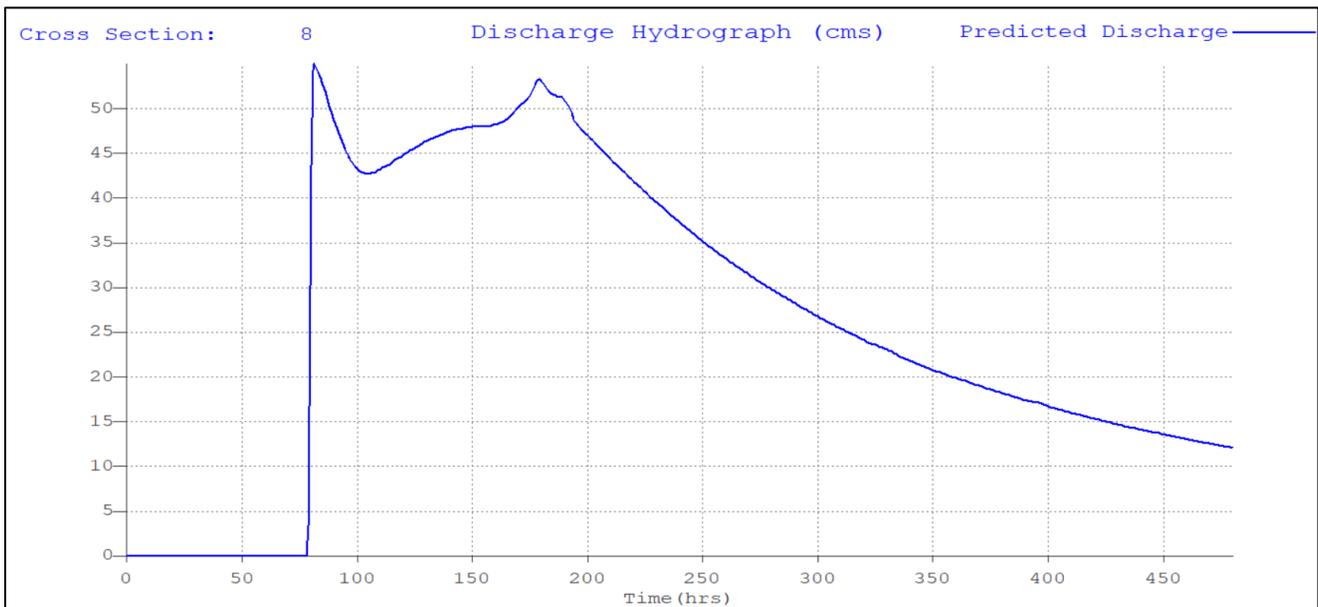
**A 23: Hydrograph at the cross-section just about Okanogan, WA showing a double peak flow, where the initial peak represents the leading edge of the debris flow, and the secondary peak represents the Lake Palmer displaced outflow. Units of flow are in cubic-meters per second. Default 40% breach scenario for the permitted CMM TSF.**
