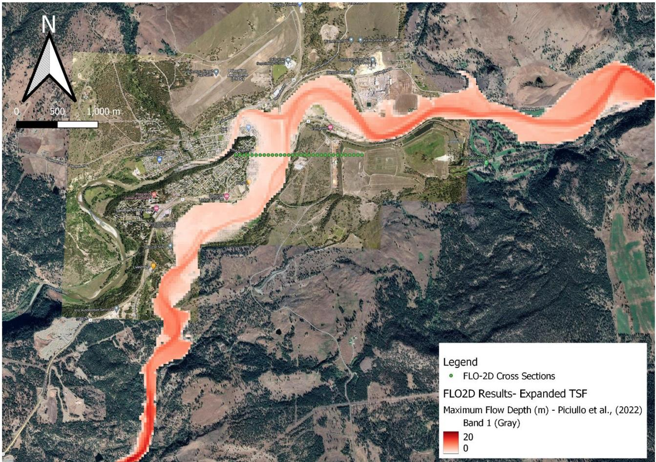
**A 25: Maximum flow depths (m) in Princeton, BC from a 23.6 Mm<sup>3</sup> breach, 12 hour duration scenario for the expanded TSF at CMM (450 Mm<sup>3</sup>), as predicted by Equation 1 in Piciullo et al., (2022). Equation 2, which uses both dam height and storage volume as predictors, is nearly identical to our 20% breach scenario.**
