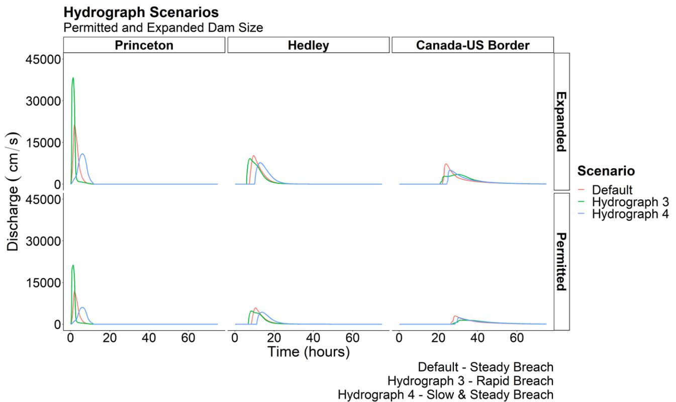
**A 18. Timeseries hydrographs of slow rise (blue), and mid rise (red), and fast rise (green) hydrographs at three cross sections along the Similkameen for the permitted dam (bottom row) and expanded dam (top row) in cubic meters per second.**
