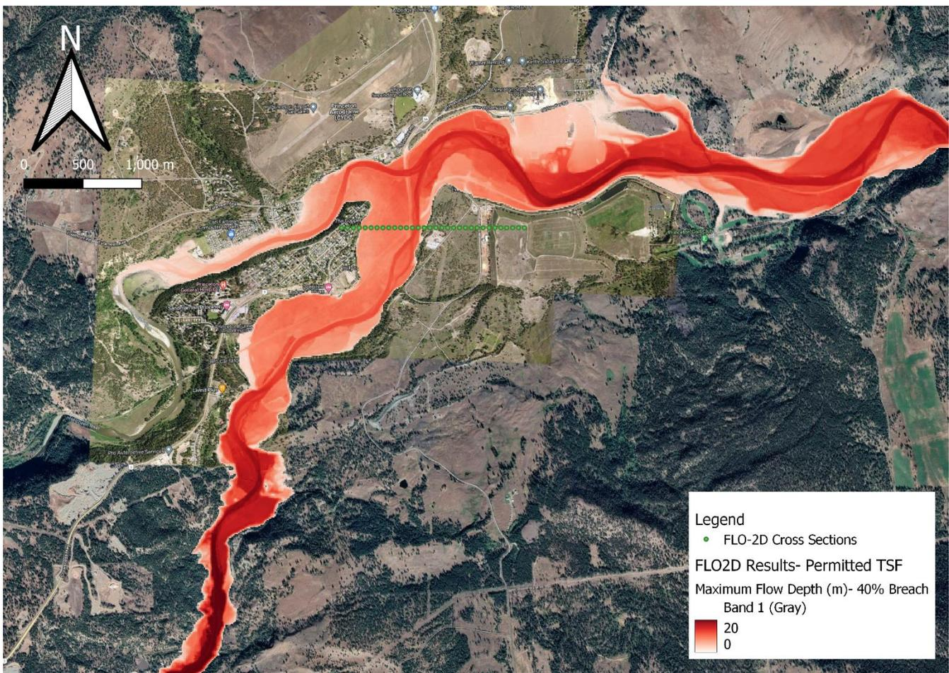
**Figure 4-2: Maximum flow depths (m) in Princeton, BC from a 40% breach, 12 hour duration scenario for the permitted TSF at CMM (250 Mm<sup>3</sup>). Debris flow is entering from bottom left and exiting at top right.**
