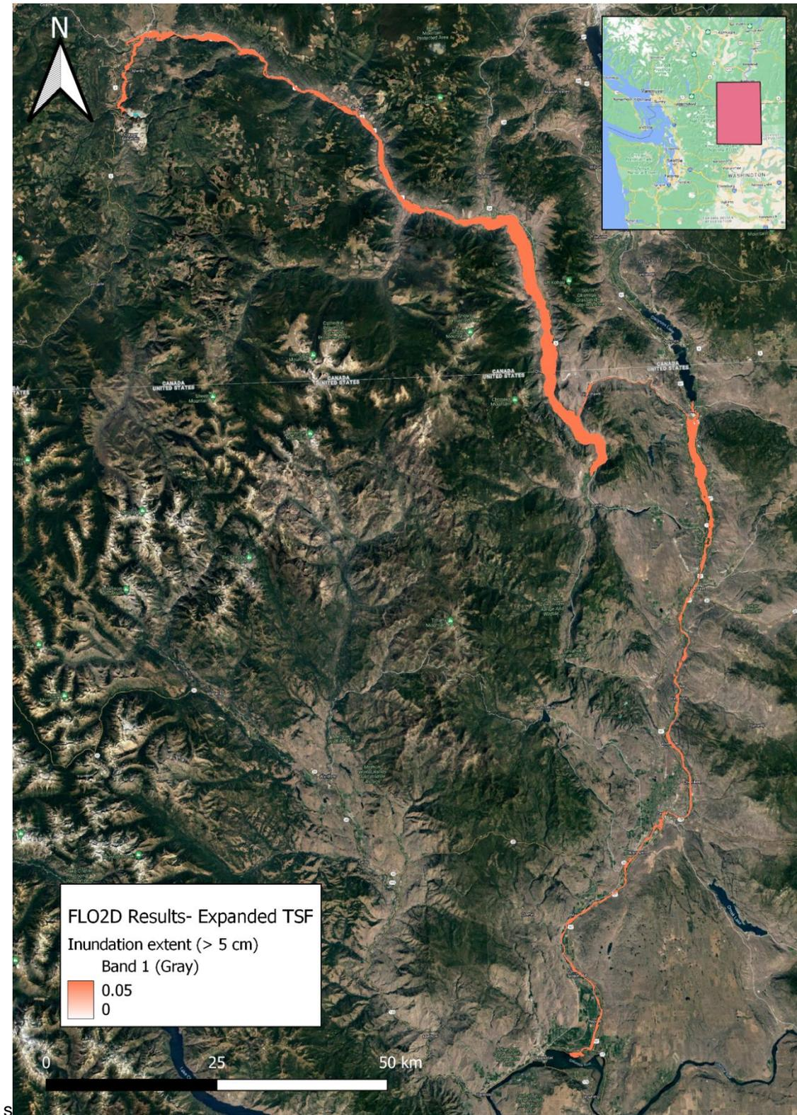
Figure 4-6: Inundation extent (> 5 cm depth) for the 40% breach, 12 hour duration scenario of the expanded TSM at CMM. 50 m spatial resolution, 480 hour simulation run time. CMM TSM is located in the upper left hand quadrant of the map, as illustrated in Figure A 20.
