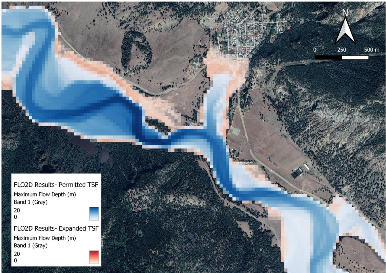
*Figure 5-2: An overlay of maximum flow depths (m) in Hedley, BC from a 40% breach, 12 hour duration scenario for the permitted TSF (250 Mm<sup>3</sup>; in blue colorbar) and the expanded TSF (450 Mm<sup>3</sup>; in red colorbar)*
